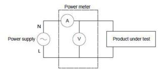
When measuring Connect the voltage measurement terminal to the a smaller current side of power supply input. Please use V+1 and Vterminal as voltage measurement terminals and I + and I- terminal as current measurement terminals.
