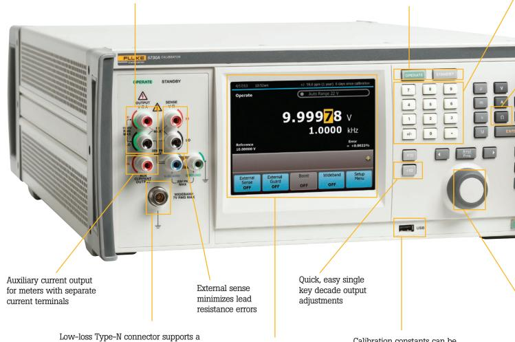
Low-loss Type-N connector supports a wideband voltage option that provides flat, low-noise alternating voltage output from 10 Hz to 30 MHz to handle RF voltmeters
