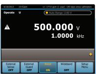
Product features like Boost and Wideband are easily activated via the five-button toolbar located at the bottom of the output screen.
