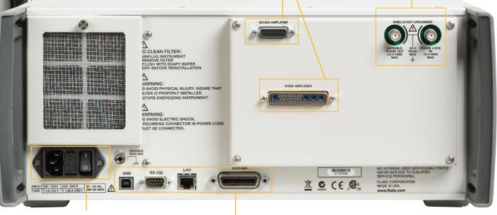
A new power switch automatically senses and adapts to the incoming mains power and frequency
