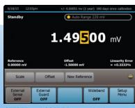
OFFSET and SCALE keys make it easy to compensate for zero offset and scale errors and permit direct display of linearity errors at any scale level.
