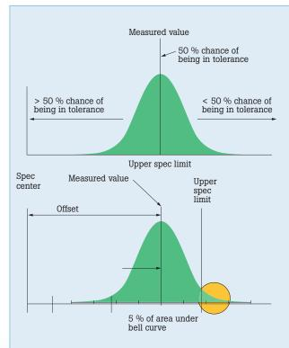
**Figure 1**. The offset of the uncertainty bell curve shows how guardbanding can give you the confidence you require in calibrations.
