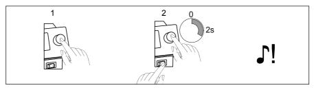
By turning the i-OP and pressing it accordingly, the station can be configured or rewritten with the factory settings.
